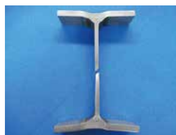
▲ After tensile testing (*fracture of base material part)
