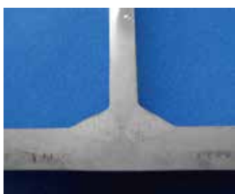
▲ Welded spot penetration state
